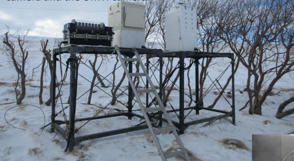
左から、多波長フォトメータ、WATEC/nightviewer camera, OMTI camera From left, multi-channel photometer, WATEC/nightviewer camera and the OMTI camera.
