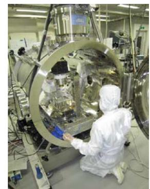
Experimental work for calibrating the medium-energy ion analyzer set in a vacuum chamber.
