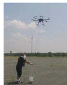
Flight experiment with a drone and an OPC.
