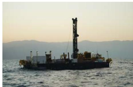
Drilling of sediment core in the Dead Sea.
