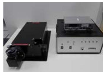
Upper: Field-of-views of the cameras in Scandinavia. Lower: (left) optical part and (right) control part and PC of the five-wavelength photometer.
