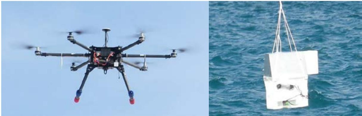
The drone used in the observation (left panel) and the lifted sonde (right panel).
