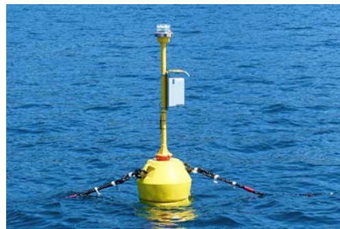
Sea-spray spectrometer probe on a mooring buoy.
