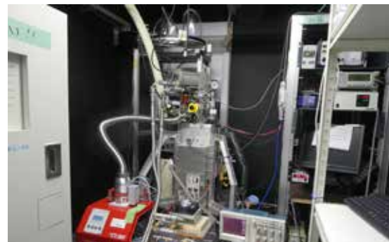
Millimeter-wave radiometer installed in Tromsø, Norway
