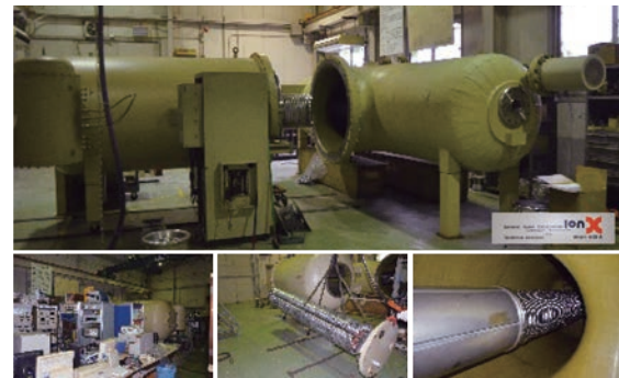
Tandron Accelerator Mass Spectrometer I that produced many 14 C important papers (Discarded in May 2021)
