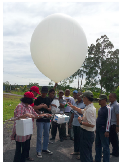
Fig. 2. The configuration of balloon and payloads (left) and the photo just before the launching the set of CFH and ECC (right) in the morning on 9 Jan. 2013.
