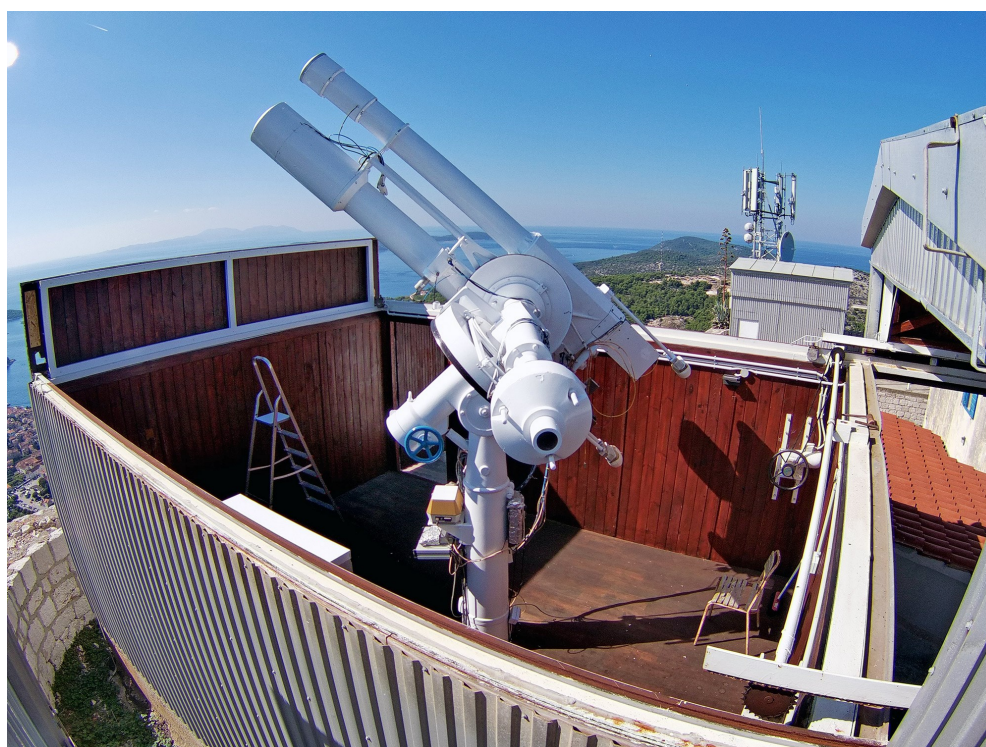
Figure 1. Double solar (white-light and H-alpha) telescope of the Hvar Observatory.
