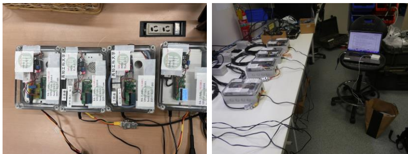
Fig. (1) Testing of INF04 sensor and datalogger in KUT at the left-hand side figure and Curtin Univ. in the right-hand side figure.
