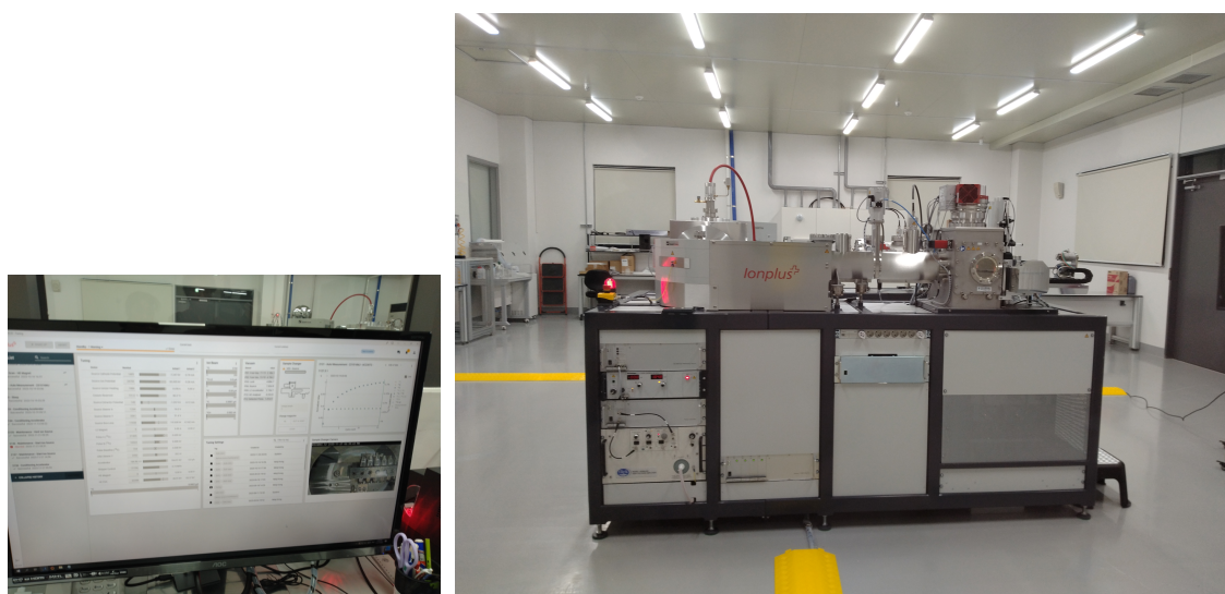
Figure 1. MICADAS, an ultra-compact ^{14}\text{C} measurement AMS system manufactured by IonPlus, installed at the National Research Institute of Cultural Properties, Korea. The photo on the left shows the PC screen used to control the MICADAS AMS system.
