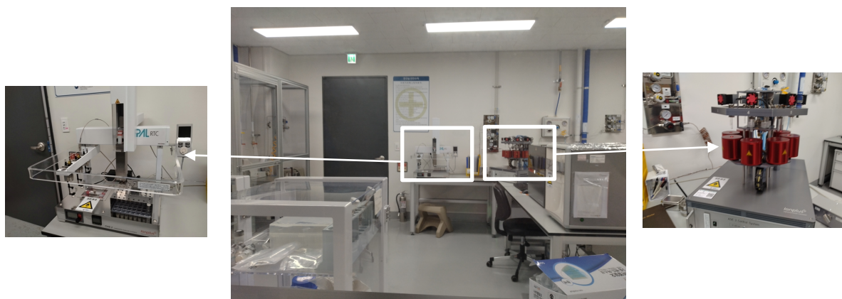
Figure 2. View of the ^{14}\text{C} sample preparation room at the National Research Institute of Cultural Heritage, Korea. On the left, automated sampling system connected to GC-MS; on the right, automated graphite equipment (AGE 3).
