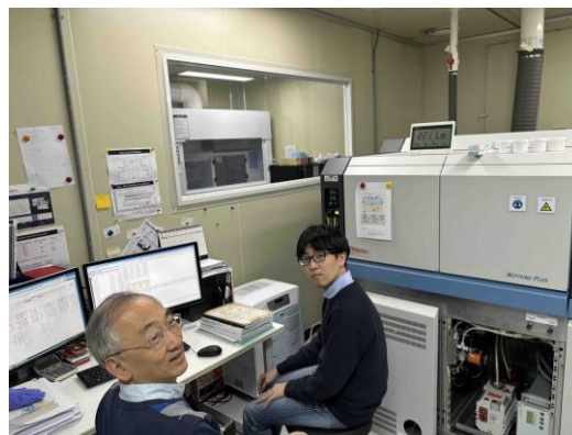
Fig. 1 Li isotope ratio measurement on volcanic rock samples by MC-ICP-MS at KIGAM (Feb. 2026).
