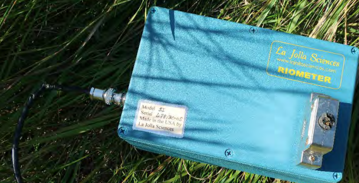
Riometer preamplifier (get out from the box, cable was cut)
