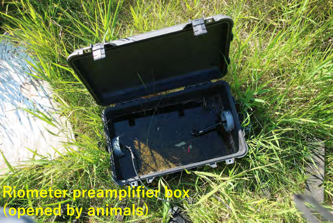
Riometer preamplifier (get out from the box, cable was cut)
