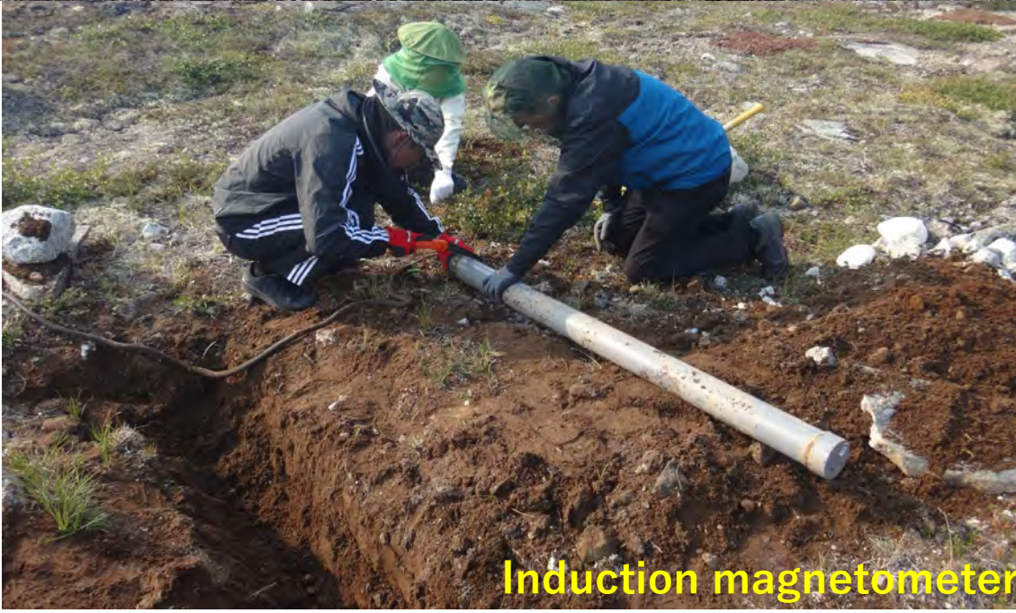
Water leak from the plastic pipe of the induction magnetometer
