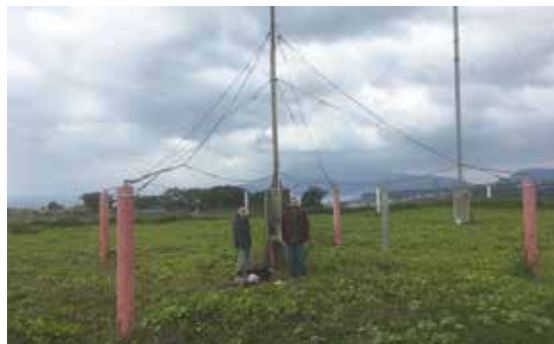
An ELF/VLF radio wave receiver installed at the Kagoshima Observatory by Georgia Tech in USA
