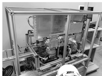
Aerosol mass spectrometer for the analysis of aerosol sample extracts.
