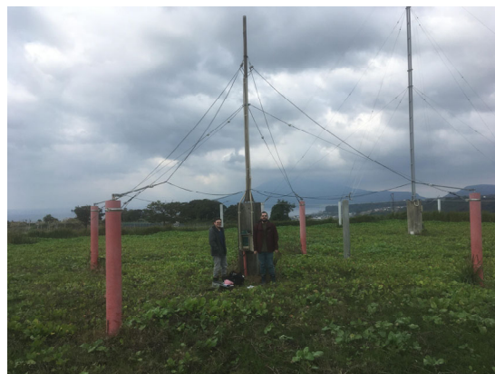
A VLF/ELF wave receiver installed at Kagoshima Observatory by Georgia Tech., USA, to observe electromagnetic waves from lightning.
