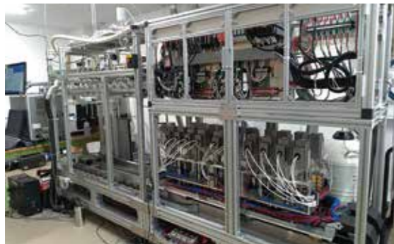
Auto Graphitization Equipment for 14 C analysis
