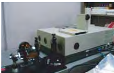
A compact FTIR measures atmospheric \text{CO}_2 concentration.
