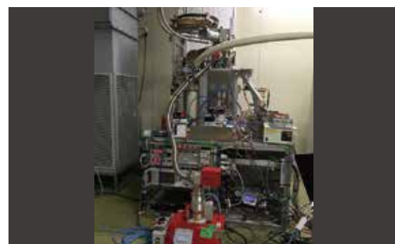
The upgraded multi-frequency millimeter-wave spectral radiometer at Syowa station, Antarctica
