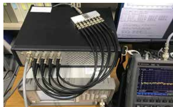
IPrototype of a digital backend for the next generation IPS observation system
