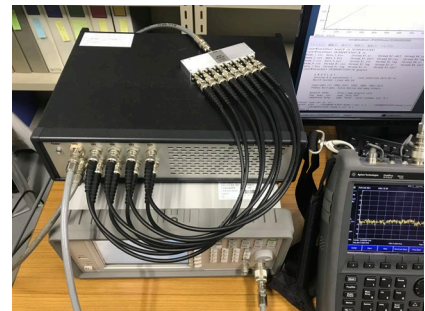
Prototype of a digital backend for the next generation IPS observation system.
