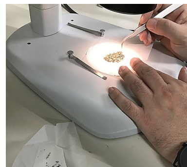
Hand-picking of olivine grains from crushed rock-sample under an optical microscope.
