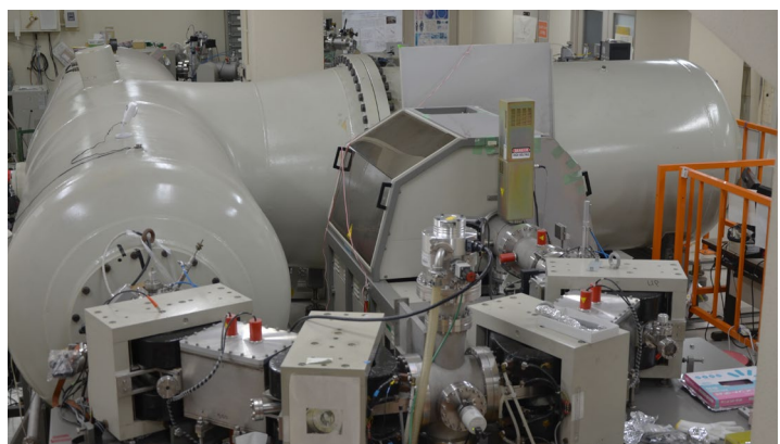
Tandatron accelerator mass spectrometer (ISEE, Nagoya Univ.).
