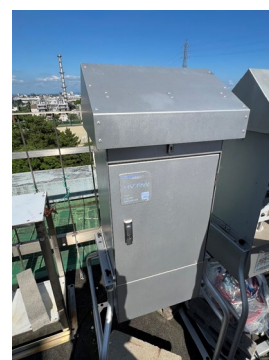
High-volume air sampler for collecting aerosol samples.
