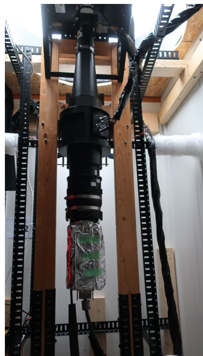
Fabry–Perot interferometer in Skibotn, Norway
