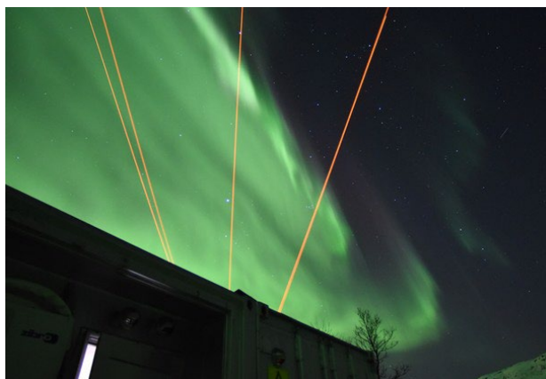
Aurora above the LIDAR container installed in Tromsø, Norway on February 28, 2025. The orange line is a laser beam (wavelength 589 nm) emitted from the LIDAR.
