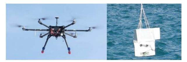
The drone used in the observation (left panel) and the lifted sonde (right panel).
