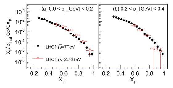
Differential cross-section of forward neutral pions measured by the LHCf with p–p collisions at $\sqrt{s}$  = 2.76 TeV and 7 TeV. The LHCf Collaboration, *Physical Review D*, 94, 032007 (2016).
