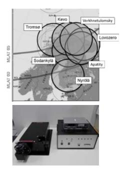
Upper: Field-of-views of the cameras in Scandinavia. Lower: (left) optical part and (right) control part and PC of the five-wavelength photometer.
