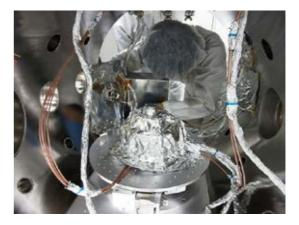
Suprathermal ion instrument for the sounding rocket experiment, set in the vacuum chamber of the beamline.
