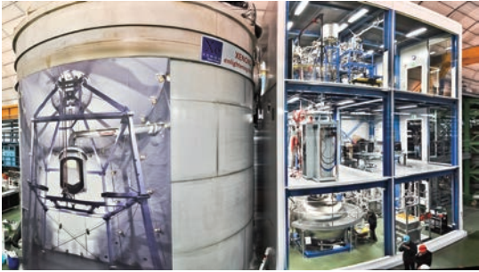
グランサッソ地下研究所の液体キセノン検出器を用いた世界最大の暗黒物質探索 XENON 実験。(写真提供：The XENON collaboration) The world's largest XENON dark matter search experiment with a liquid xenon detector in the Gran Sasso underground laboratory. (Credit: The XENON Collaboration)
