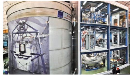
グランサッソー地下研究所の液体キセノン検出器を用いた世界最大の暗黒物質探索 XENON 実験。(写真提供：The XENON collaboration) The world's largest XENON dark matter search experiment with a liquid xenon detector in the Gran Sasso underground laboratory. (Credit: The XENON Collaboration)
