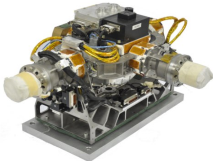
Figure 1. The instrument of FY-3C Solar Irradiance Monitor-II.
