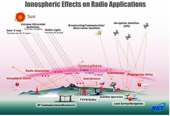
Figure 2. Effects of Ionosphere on Communication and Navigation (credit: http://wdc.nict.go.jp/IONO/index\_E.html).
