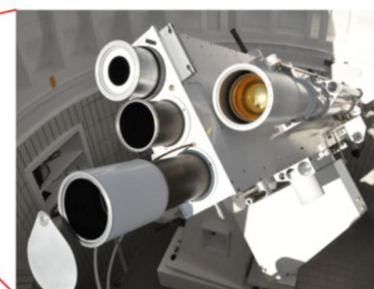
Figure 1. Kanzelhöhe Observatory (left) and its solar patrol telescope consisting of four refractors observing the Sun in H \alpha , Ca II K, and white light (right).
