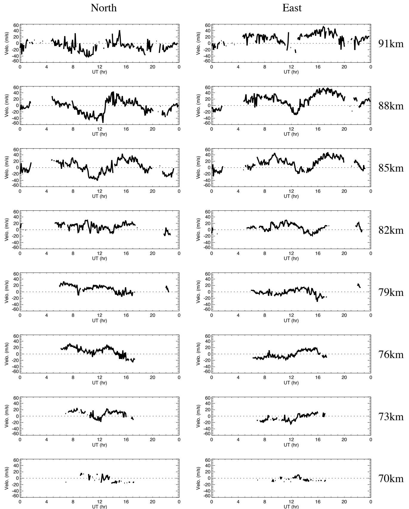
Wind data obtained by MF radar at Tromsoe on April 12, 2012
