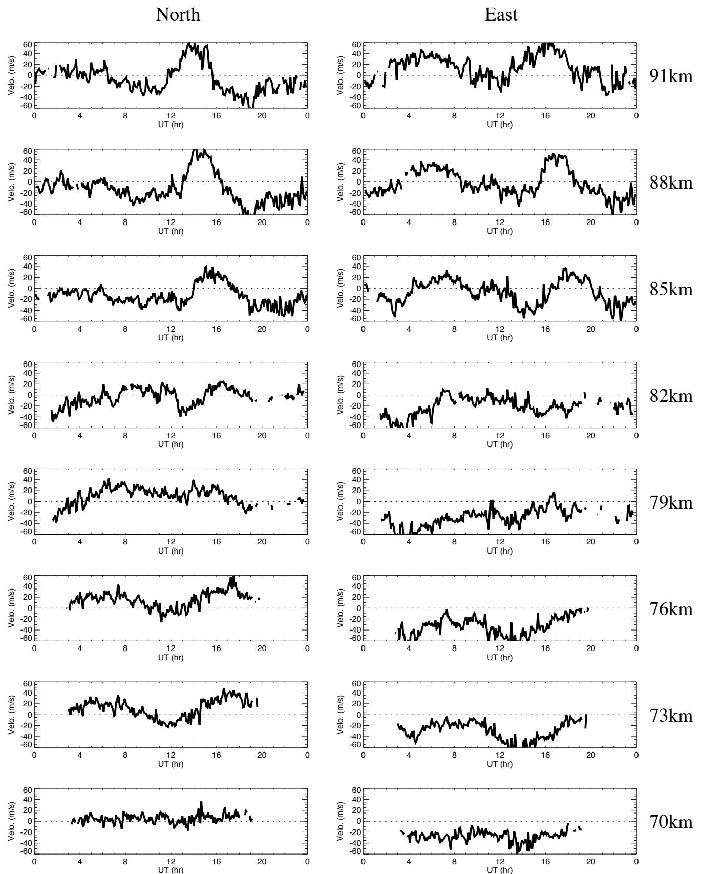
Wind data obtained by MF radar at Tromsoe on July 25, 2006
