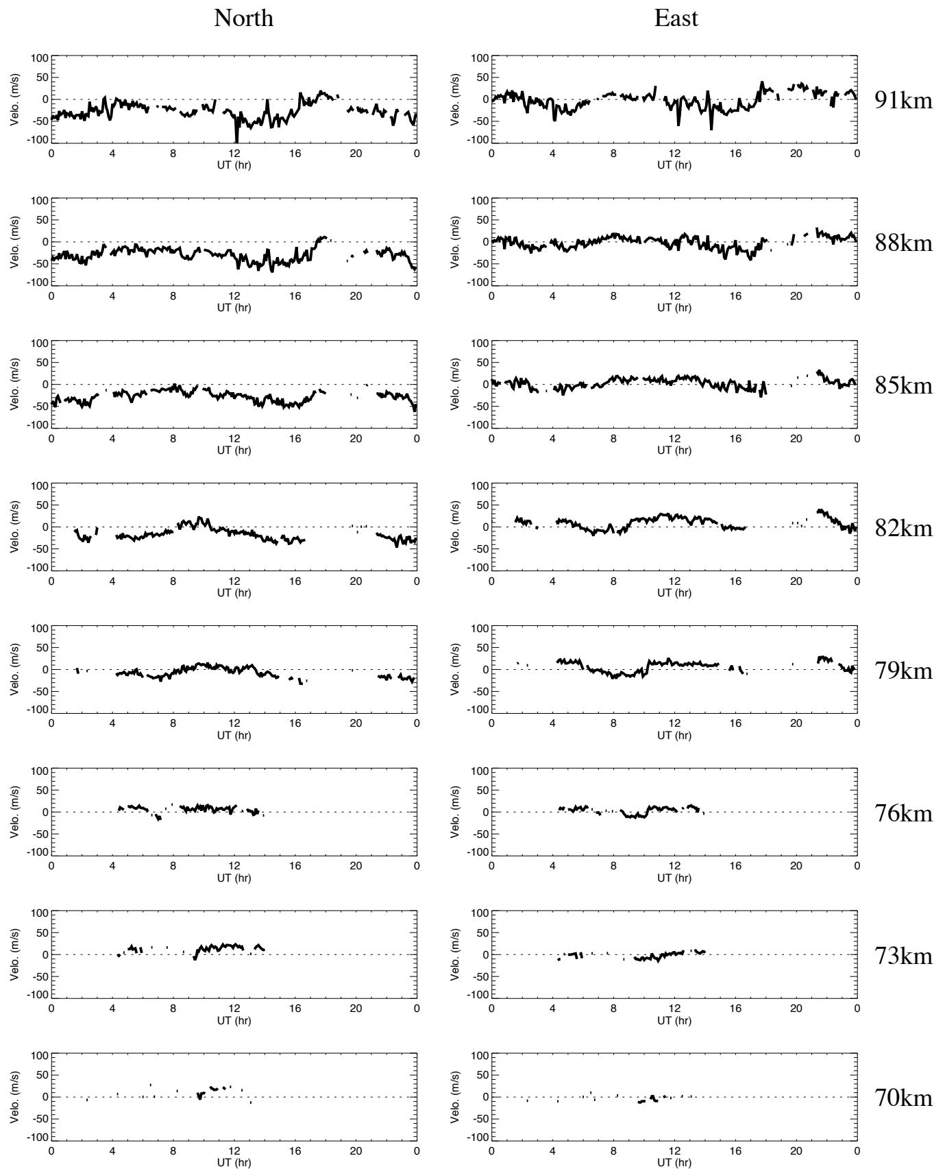
Wind data obtained by MF radar at Tromsoe on April 4, 2015
