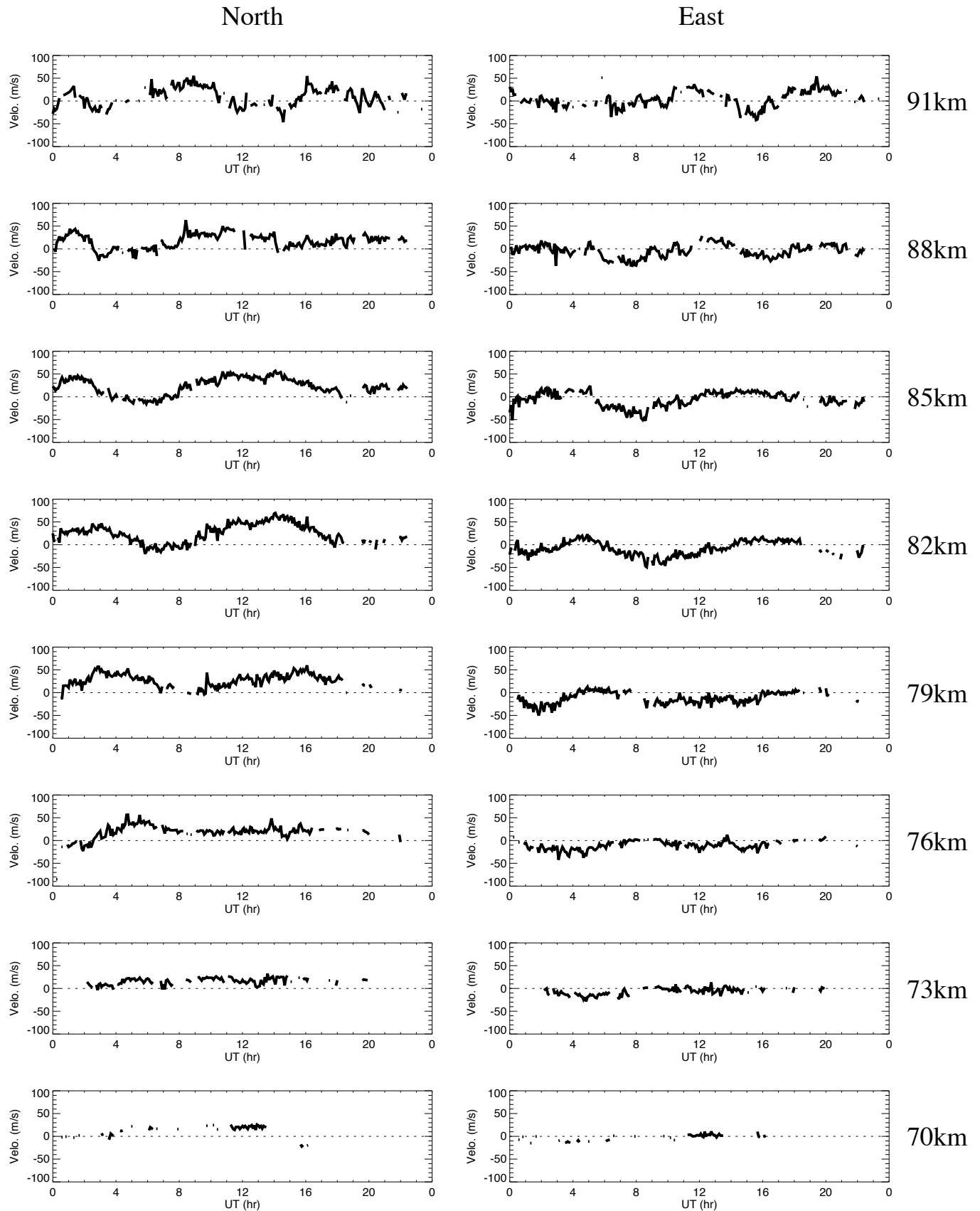
Wind data obtained by MF radar at Tromsoe on April 12, 2015
