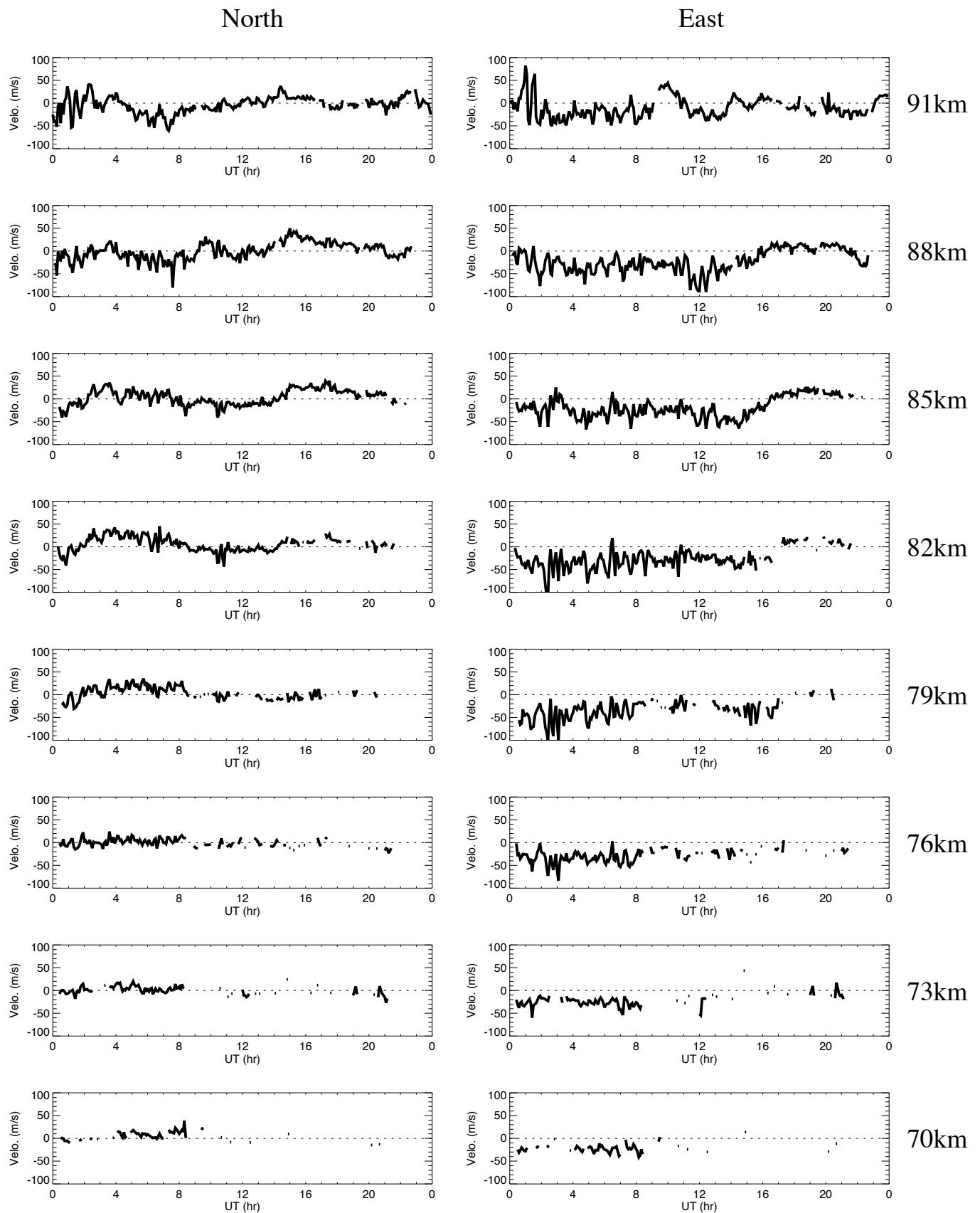
Wind data obtained by MF radar at Tromsoe on June 30, 2016
