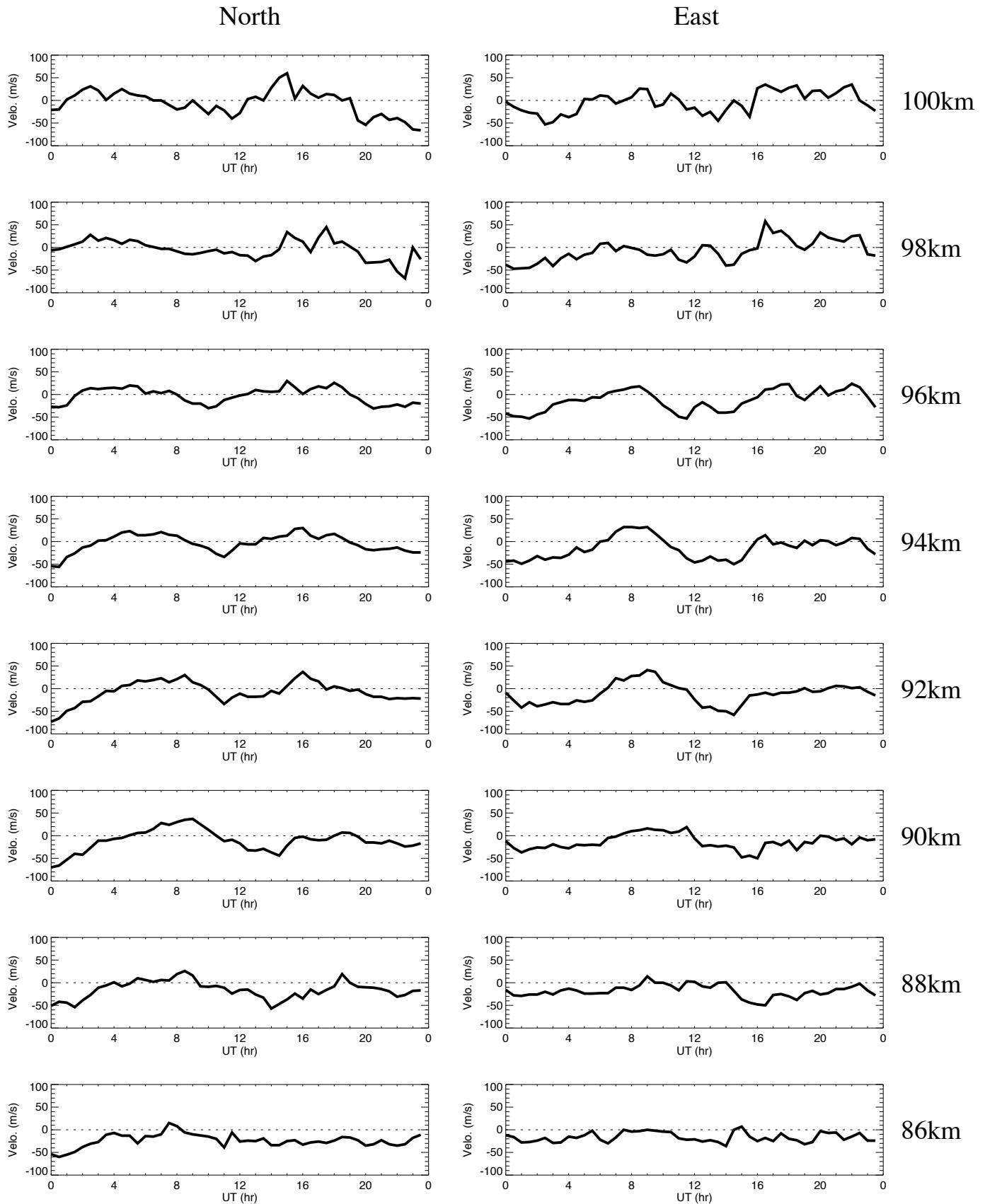
Wind data obtained by meteor radar at Alta on March 13, 2016
