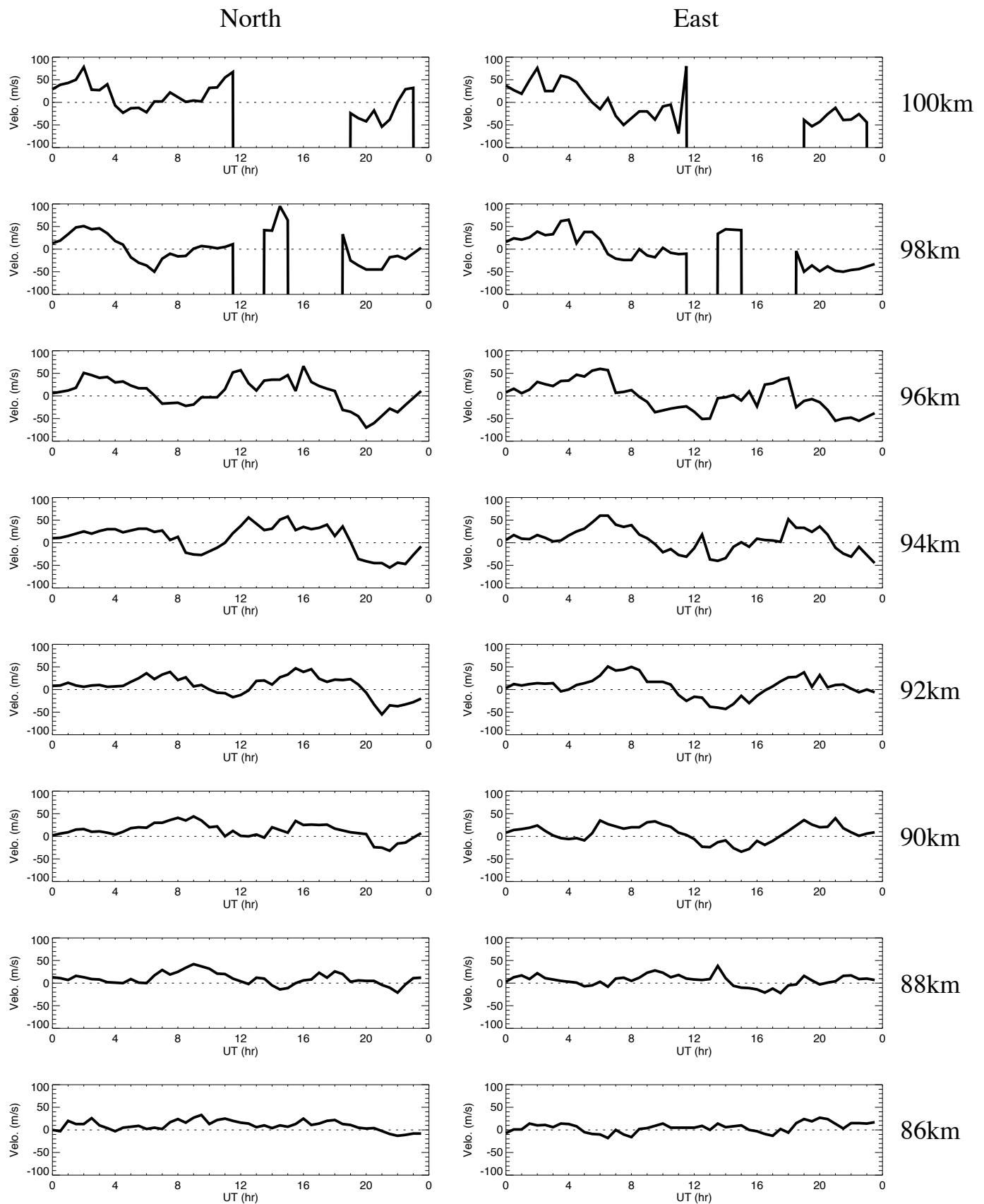
Wind data obtained by meteor radar at Alta on March 18, 2016
