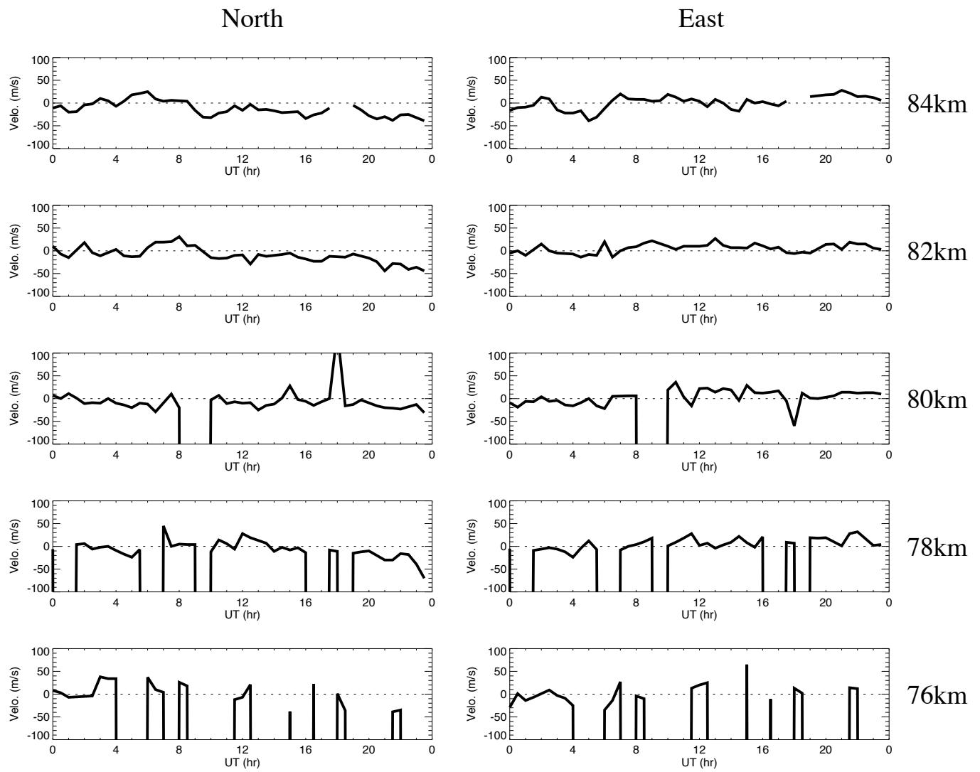
Wind data obtained by meteor radar at Alta on March 13, 2016
