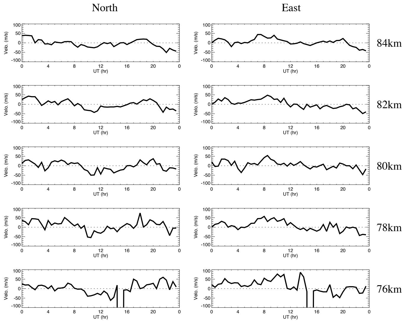
Wind data obtained by meteor radar at Alta on November 20, 2016
