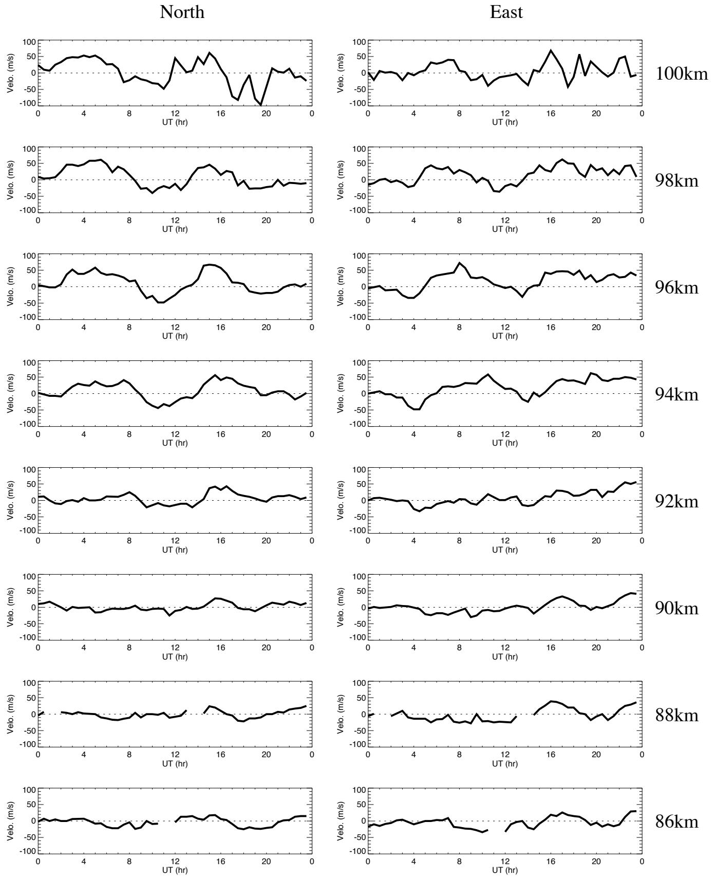
Wind data obtained by meteor radar at Alta on November 16, 2016
