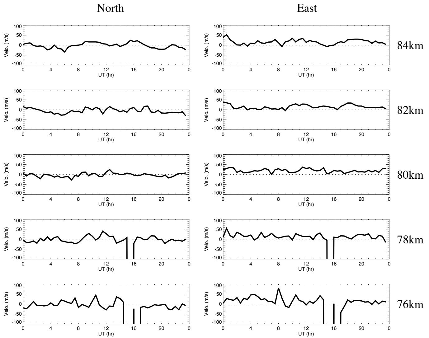
Wind data obtained by meteor radar at Alta on November 18, 2016
