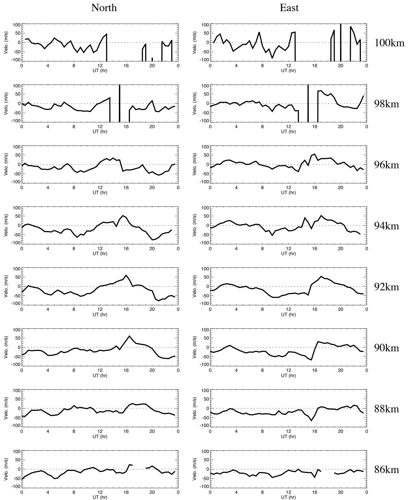
Wind data obtained by meteor radar at Alta on June 3, 2017
