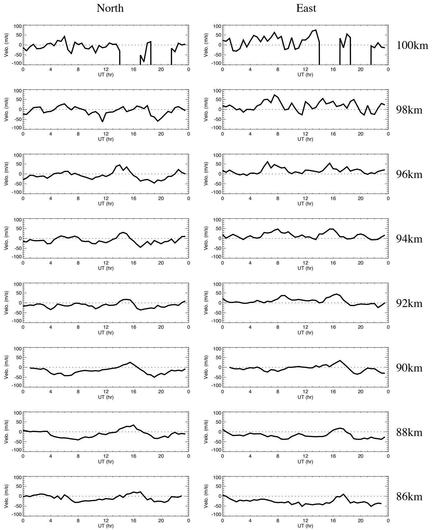
Wind data obtained by meteor radar at Alta on June 30, 2017
