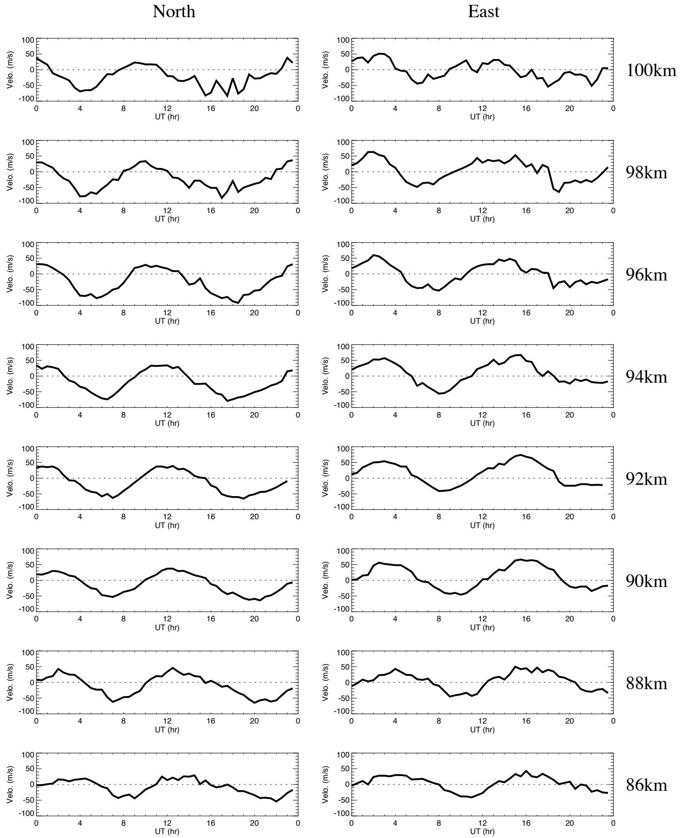
Wind data obtained by meteor radar at Alta on September 25, 2017
