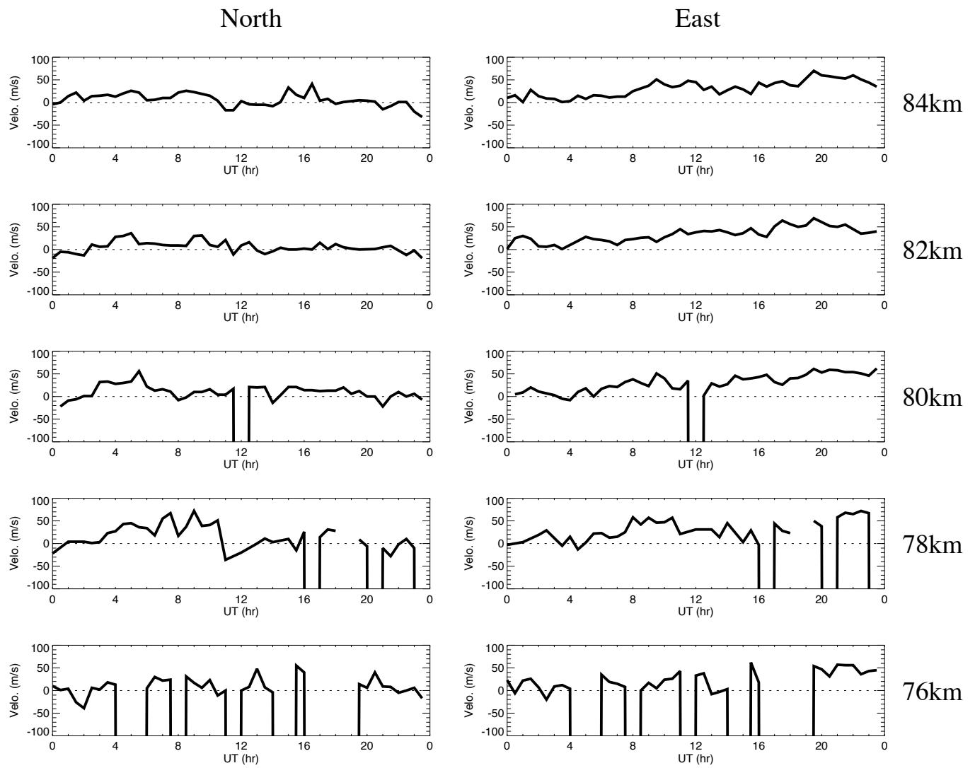
Wind data obtained by meteor radar at Alta on February 13, 2018
