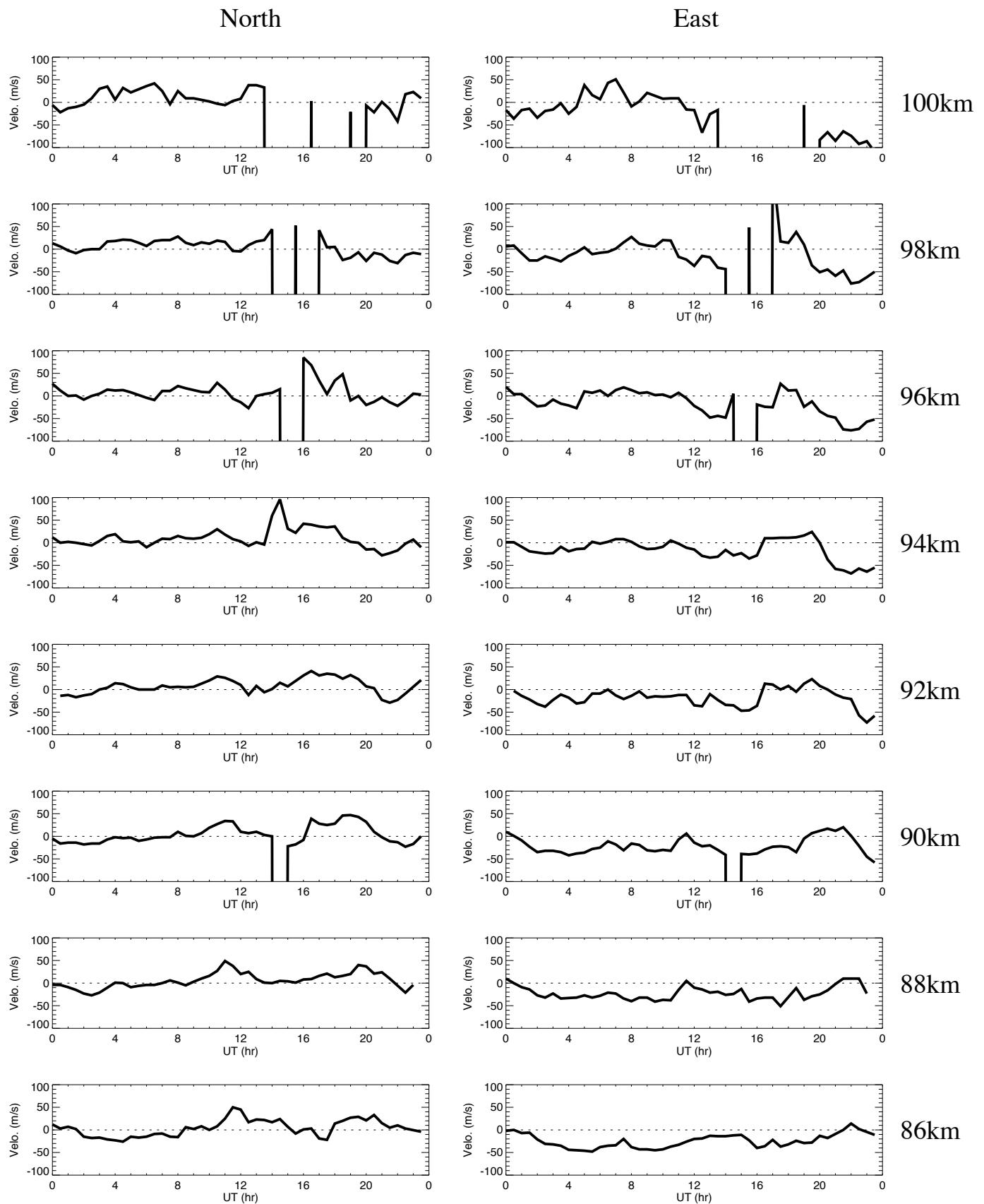
Wind data obtained by meteor radar at Alta on February 15, 2018
