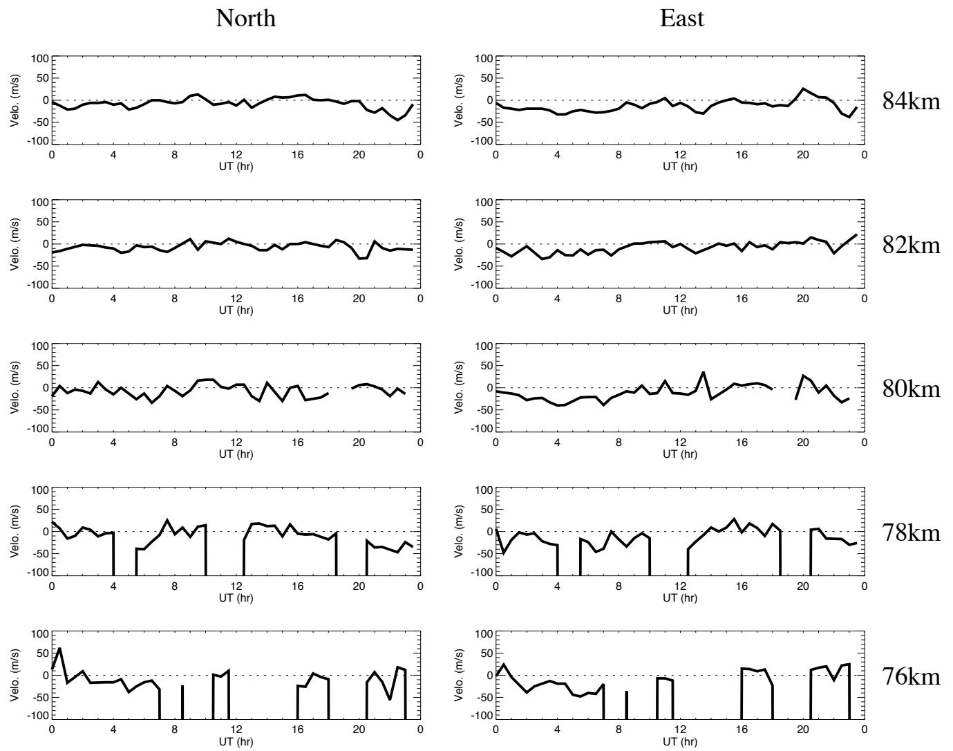
Wind data obtained by meteor radar at Alta on May 4, 2018
