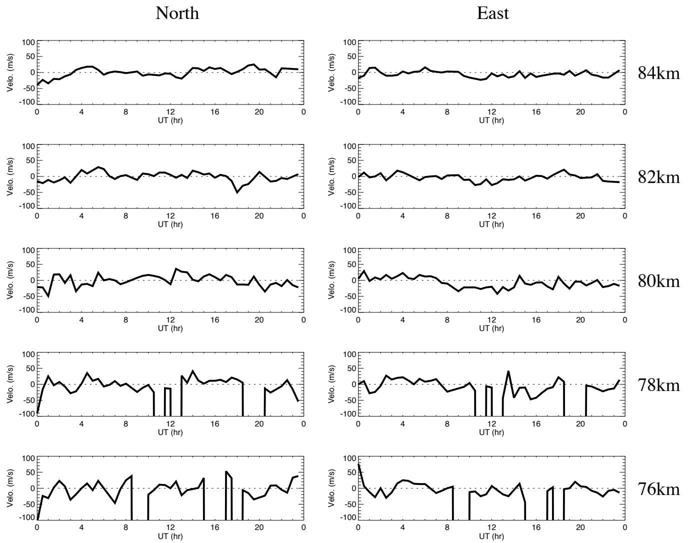
Wind data obtained by meteor radar at Alta on May 23, 2018
