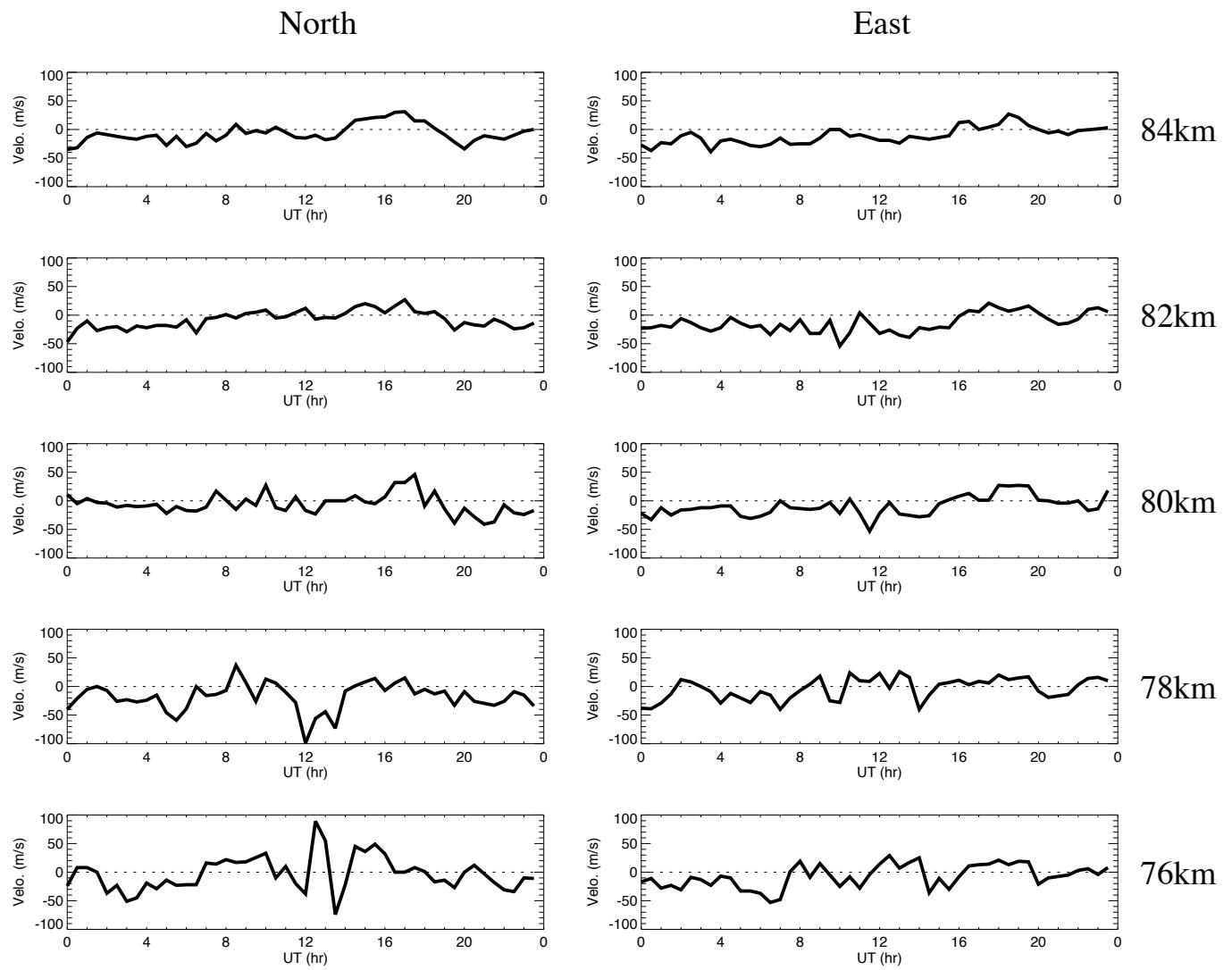
Wind data obtained by meteor radar at Alta on July 7, 2018
