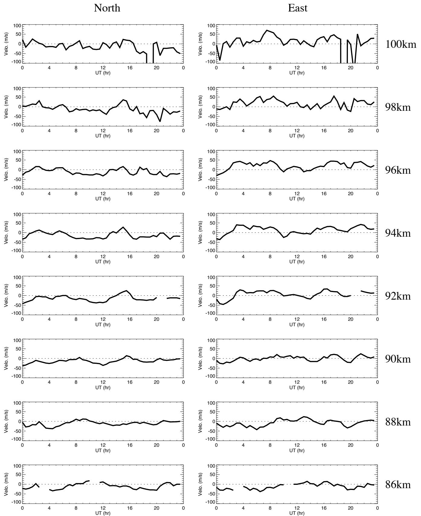
Wind data obtained by meteor radar at Alta on July 27, 2018
