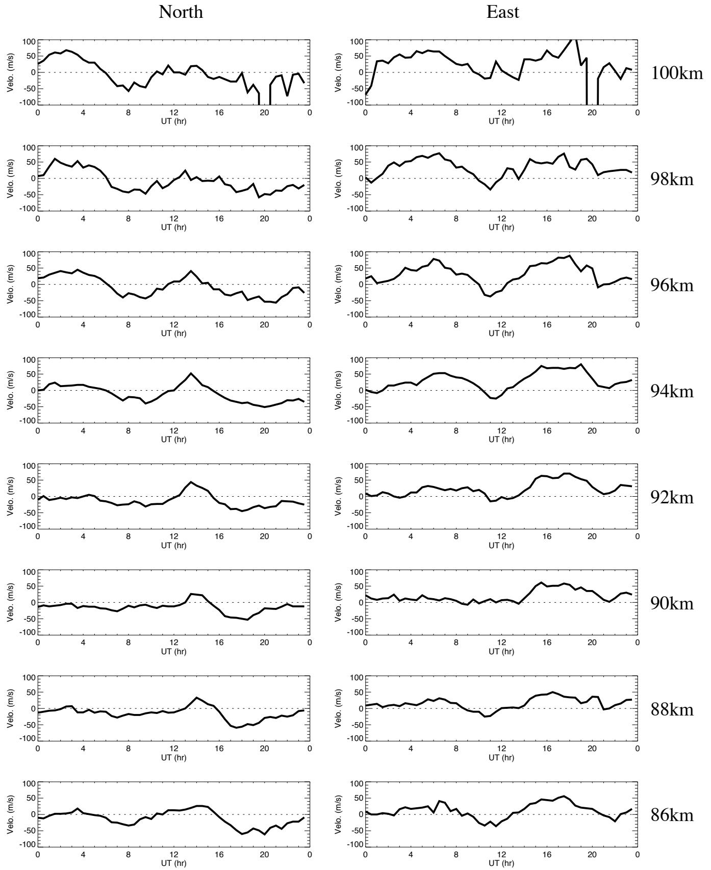
Wind data obtained by meteor radar at Alta on August 28, 2018
