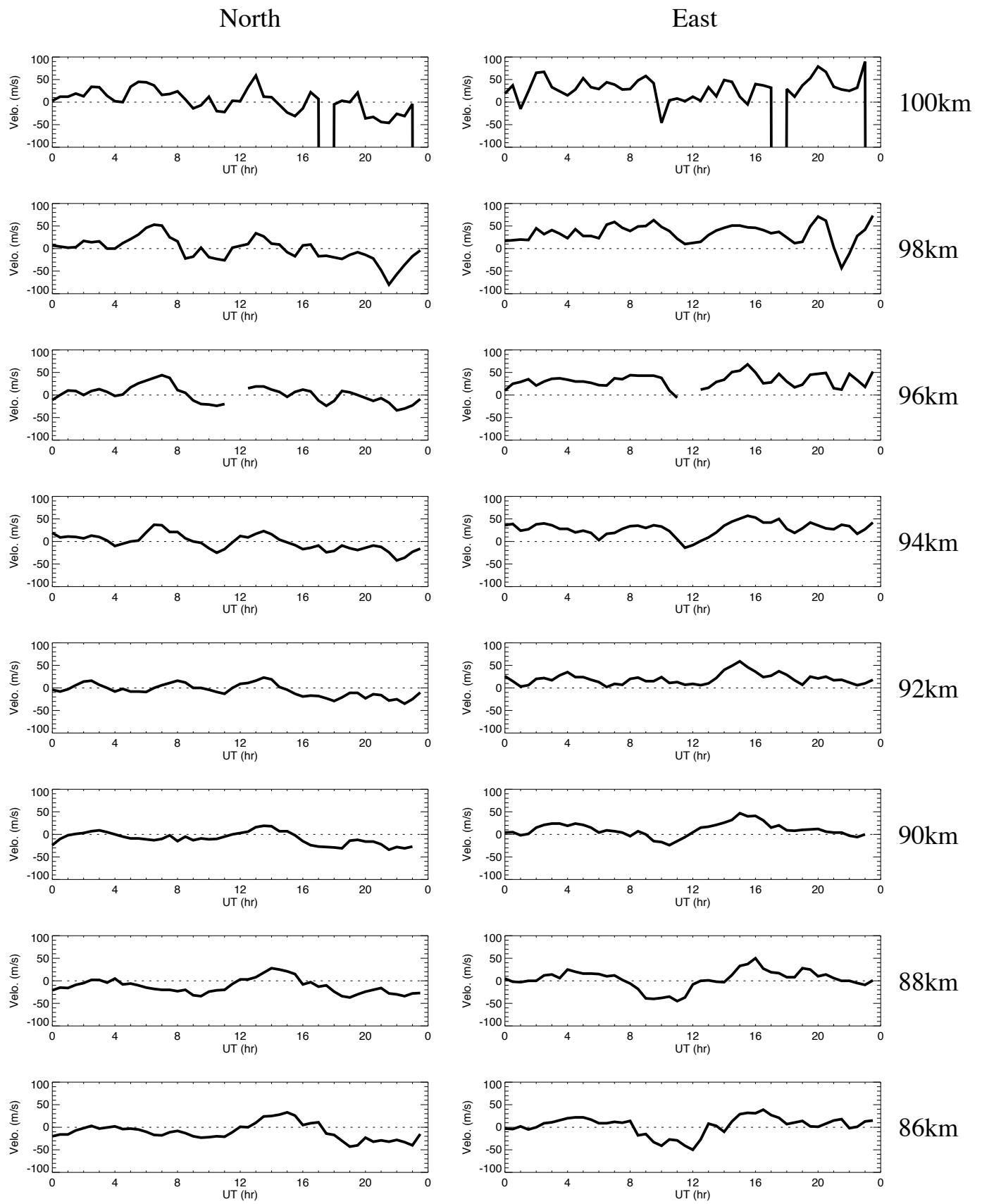
Wind data obtained by meteor radar at Alta on August 17, 2018
