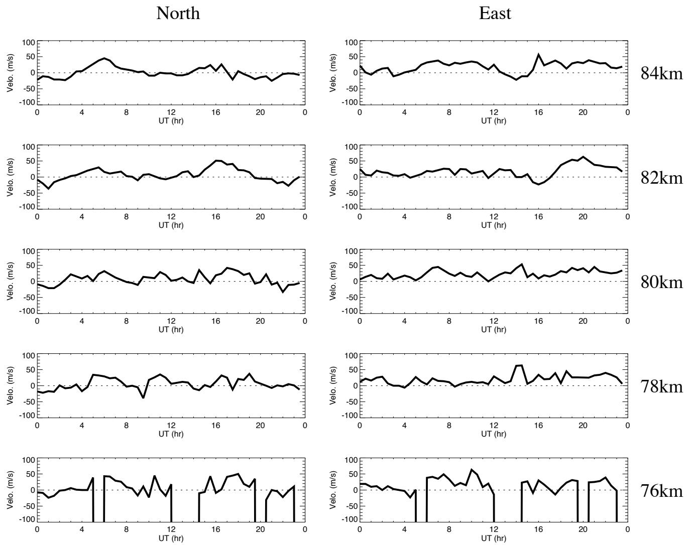
Wind data obtained by meteor radar at Alta on March 19, 2019
