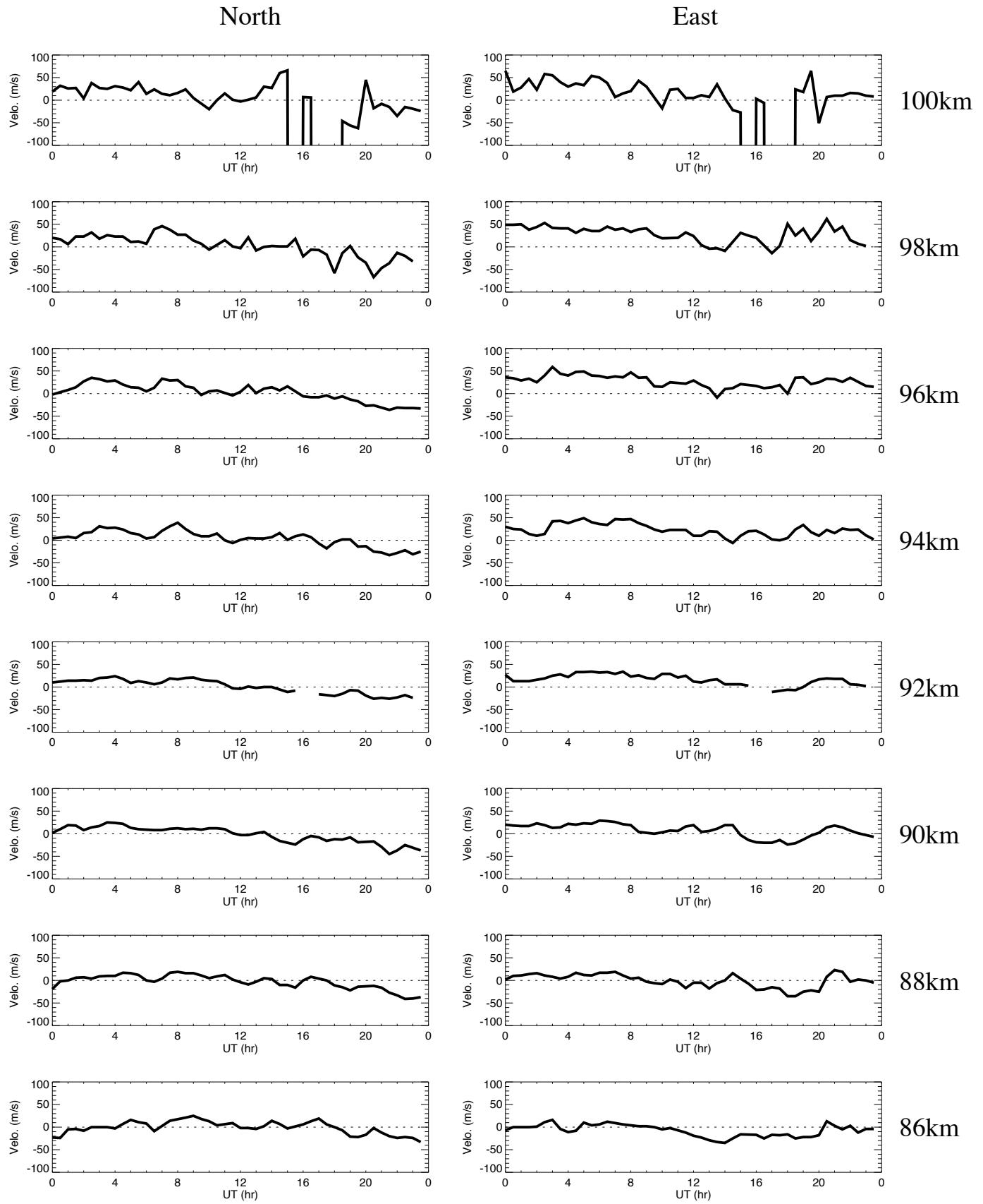
Wind data obtained by meteor radar at Alta on June 21, 2019
