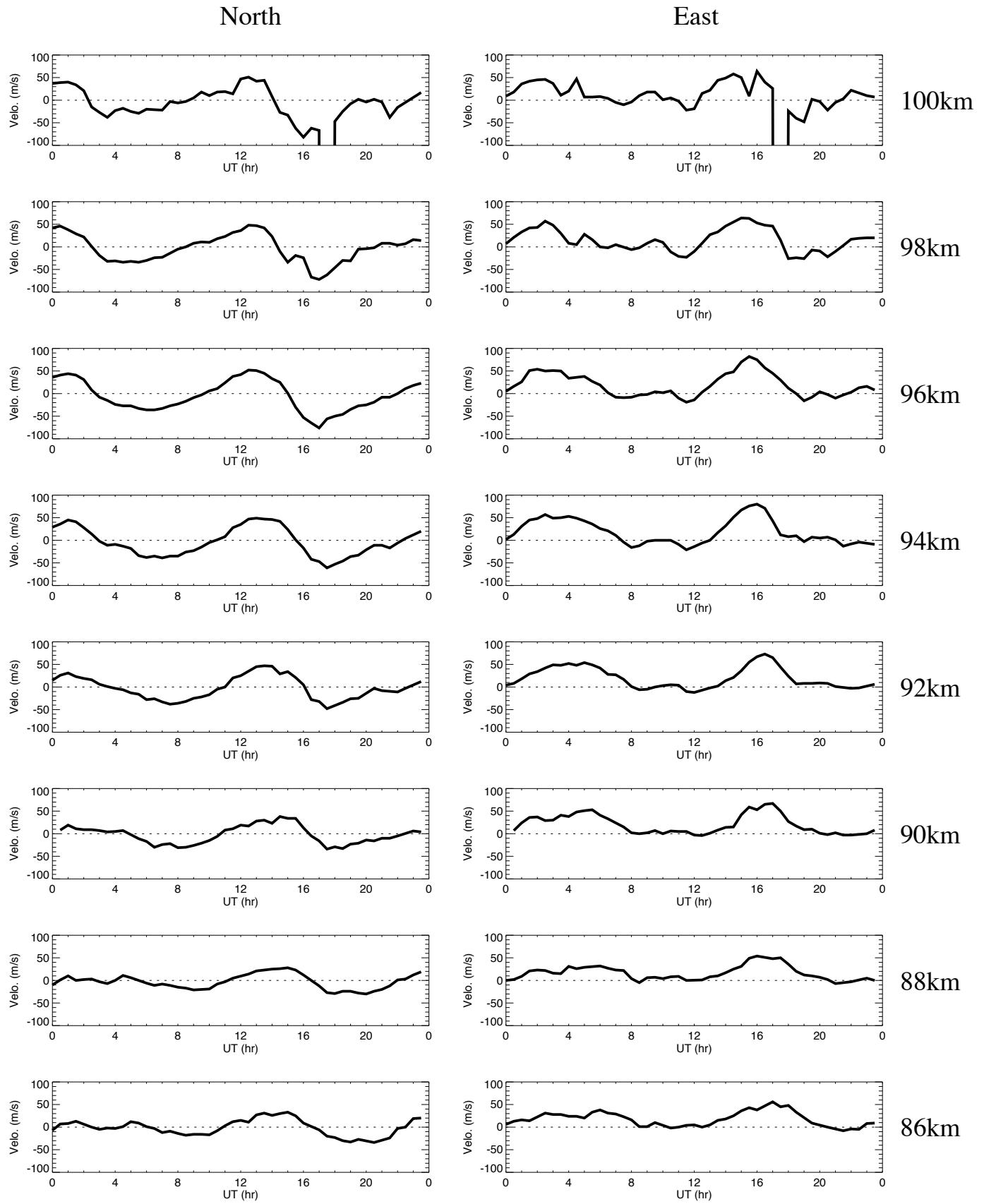
Wind data obtained by meteor radar at Alta on September 19, 2020
