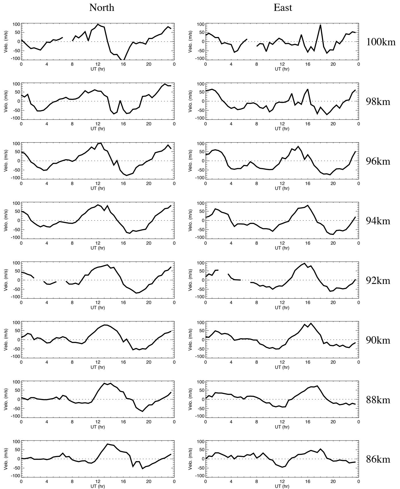
Wind data obtained by meteor radar at Alta on September 26, 2020
