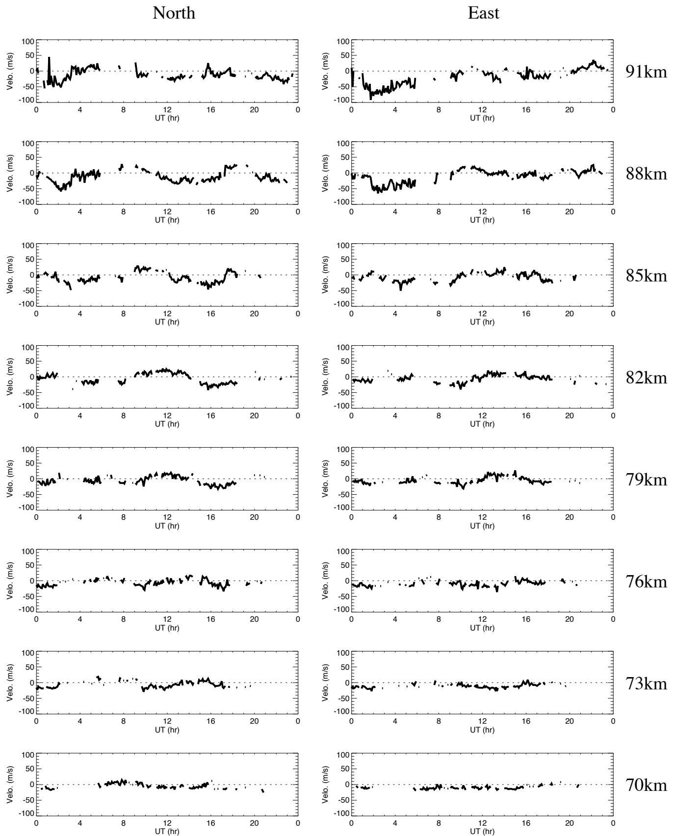
Wind data obtained by MF radar at Tromsoe on April 28, 2017
