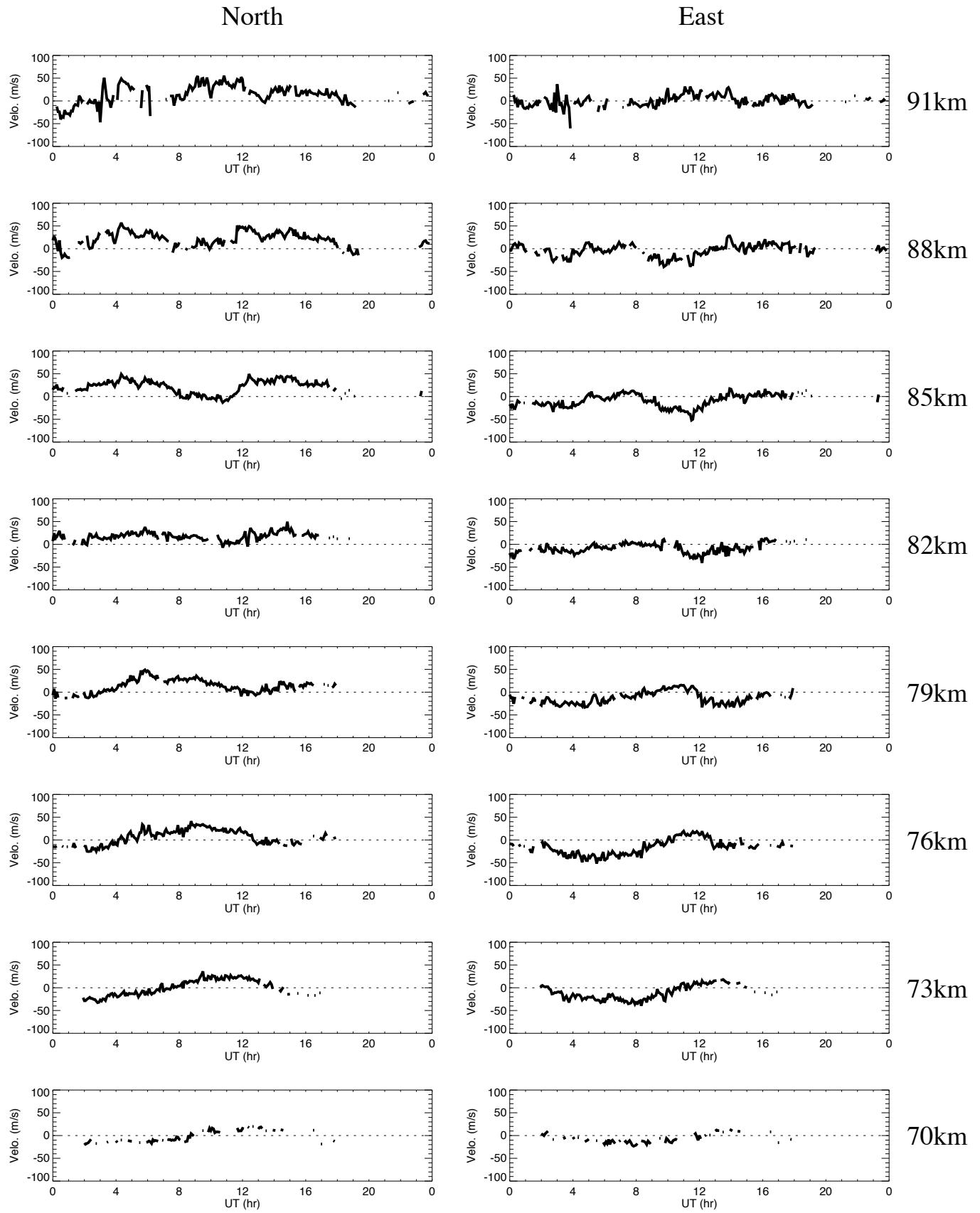
Wind data obtained by MF radar at Tromsoe on April 16, 2017
