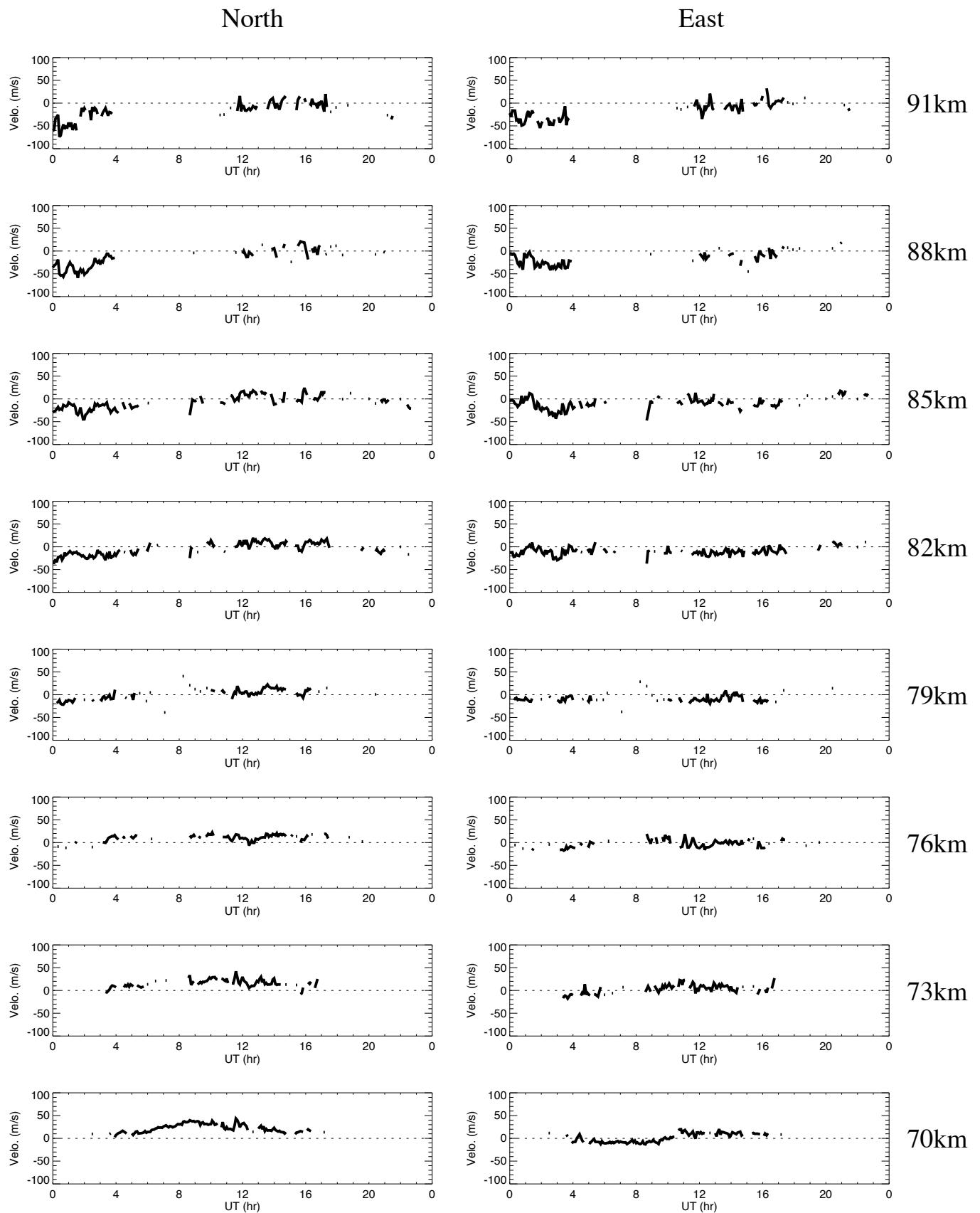
Wind data obtained by MF radar at Tromsoe on April 3, 2017
